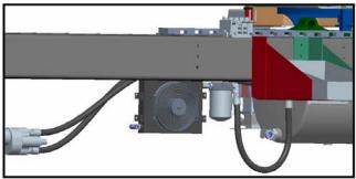
The hydraulic pump and reservoir were located in the front of the semi-tractor since it would be easier to have all the hydraulic components centrally located.
